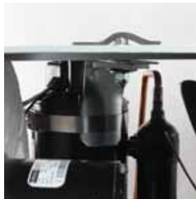
Compressor is bracketed at top and bottom to minimize vibration and movement
